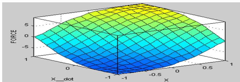
Figure 5. Surface viewer for cart controller
