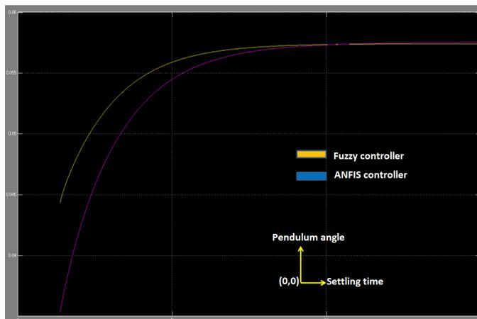
Figure 13. Simulation response for pendulum angle ( $\theta$ )
