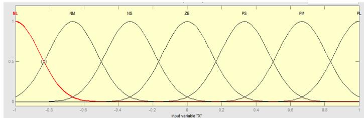
Figure 4. Membership functions designed for cart controller
